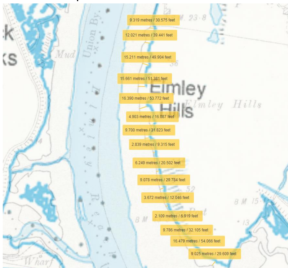
Figure 5: Example of historic retreat analysis at Elmley Hills comparing 1888-1913 OS map with recent 2015 OS map
